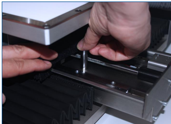
Fig. 54: Pulling out the bolt
