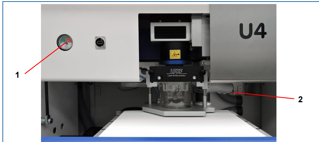
Fig. 26: Displays and control elements in the processing area
