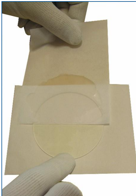
Fig. 160: Cleaning the protection glass
