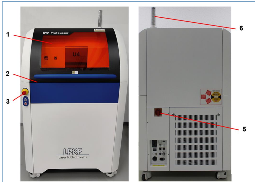
Fig. 2: System with safety devices
