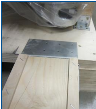
Fig. 16: Placing the transport ramps
