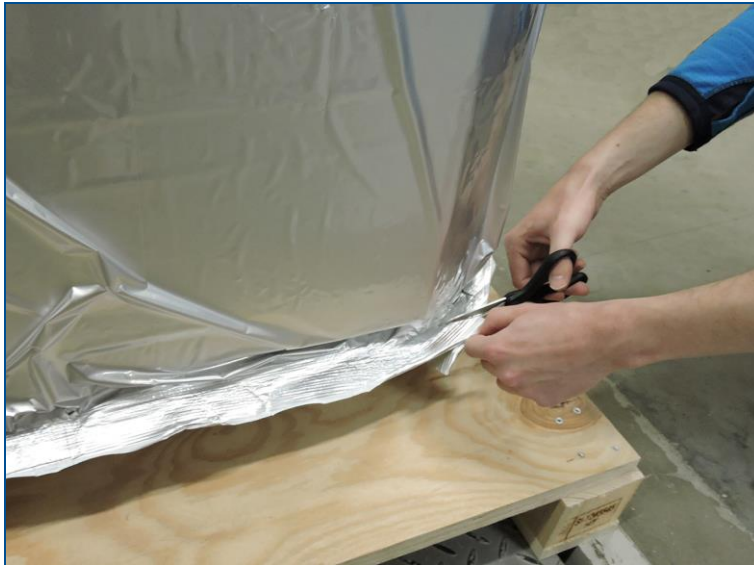
Fig. 13: Cutting off the welded parts of the foil
