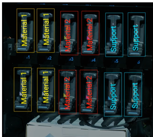
Figure 4-6 Material cabinet setup for Long Print and High Quality High Speed modes
