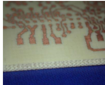
Rogers 4730G3 laser etch, cut and drill
