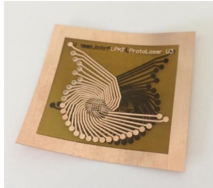
DuPont™ Pyralux® TK 127512R (3 mil thick) double sided w/ ProtoLaser U3 or U4
