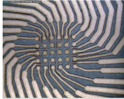
Taconic RF-35TC 1oz 85µm traces
