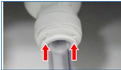
Fig. 92: Ring on drain valve
