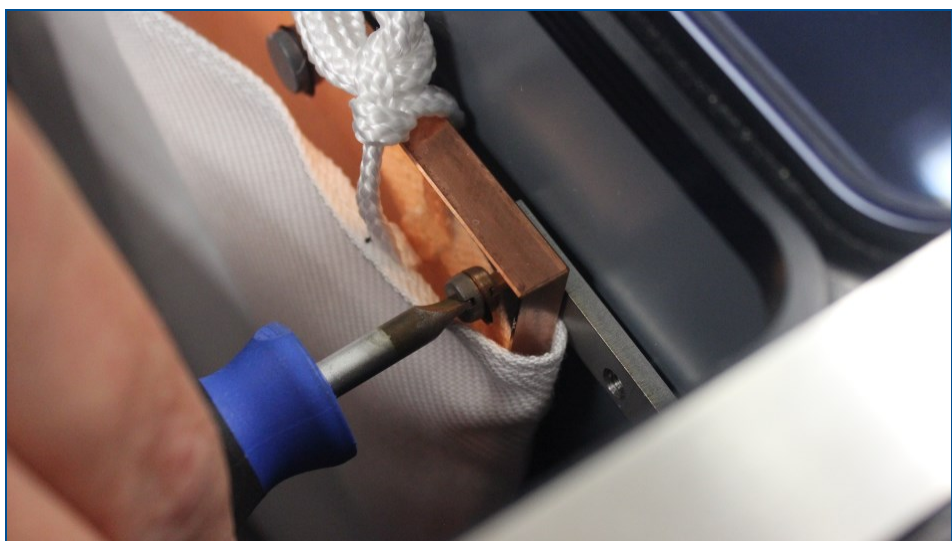
Fig. 26: Fastening the anode to the titan bracket
