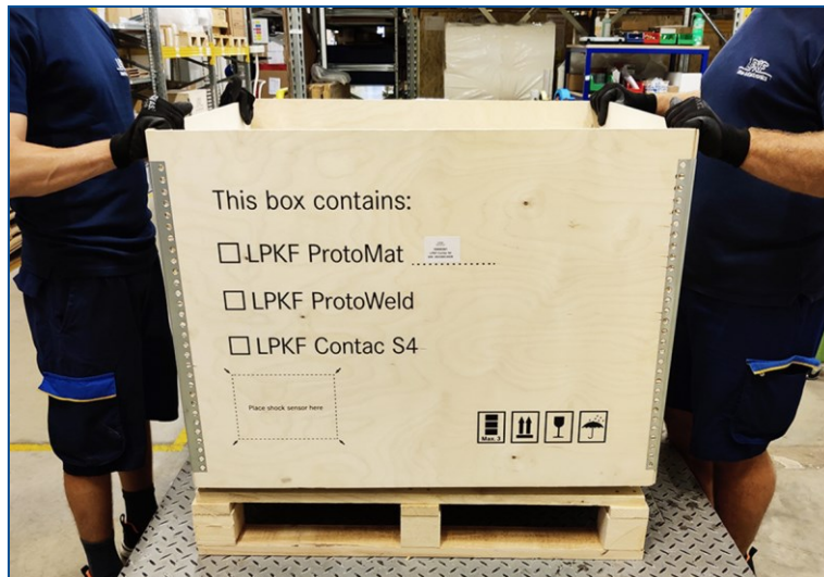
Fig. 16: Pulling the transport box upwards
