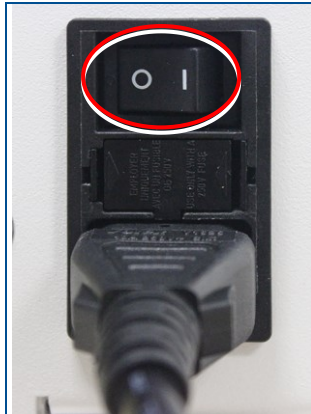
Fig. 94: Main switch off
