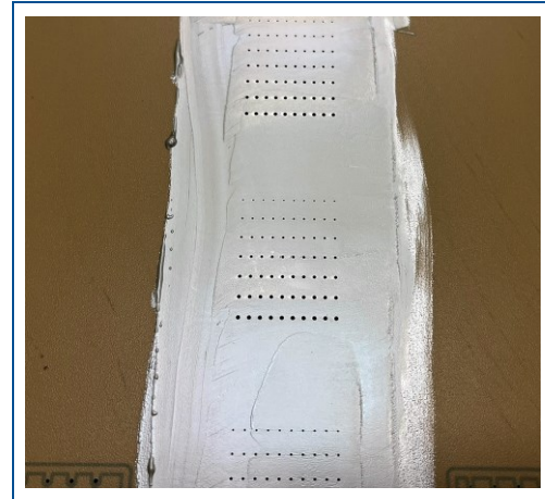
Fig. 15: Drill holes after vacuum
