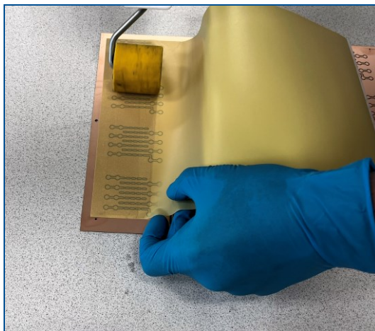
Fig. 3: Applying the protective film with the foam rubber roller
