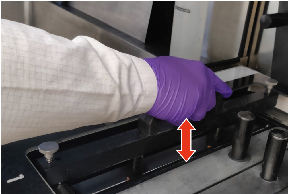
Figure 8: Lift and knock the PCB holder 8–10 times to remove air bubbles from drilled holes.
