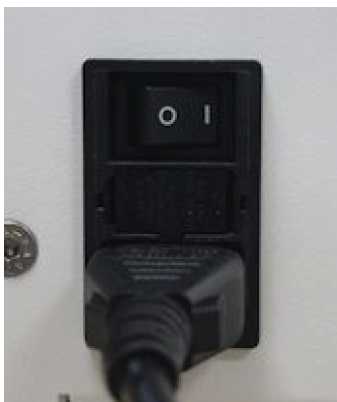
Figure 1: Main switch in the On position.
