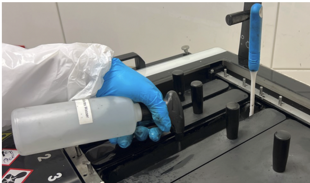
Figure 18: Final de-ionized-water rinse during authorized cleaning of Tank 3.
