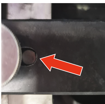
Figure 7: Correct engagement of the tank pin and PCB-holder opening.
