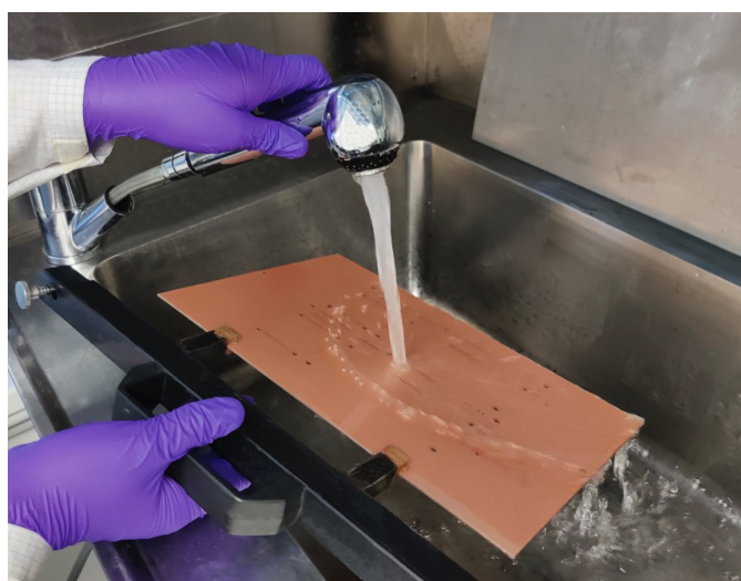
Figure 5: Rinse the mounted PCB for at least 30 seconds before processing.
