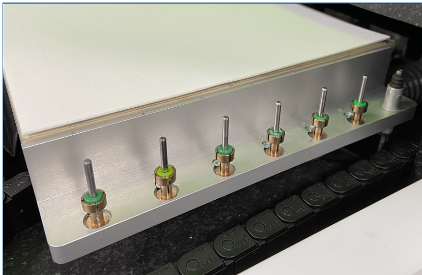
Fig. 236: Loaded tool magazine (example)
